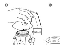
c. Firmly tighten the top and lower pots (Figure 1), and place the Moka Pot on the Heating Plate (Figure 2).
