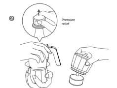
b. Lift the pressure valve to release the pressure, unscrew the Moka Pot, discard the coffee capsules (Figure @). Wash thoroughly the upper and lower pots.
